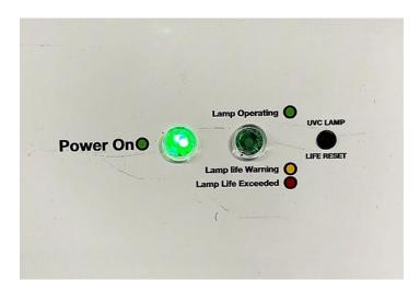
a. If all the connections are correct and the outlet is tested to verify the unit is receiving power but the "Power On" LED still isn't illuminated, turn your unit off and contact an Air Sniper representative.
