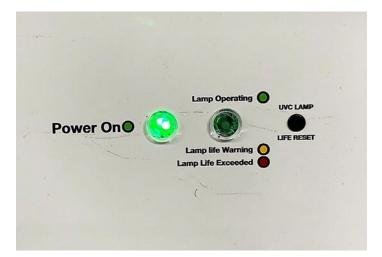
a. If all the connections are correct and the outlet is tested to verify the unit is receiving power but the "Power On" LED still isn't illuminated, turn your unit off and contact an Air Sniper representative.
