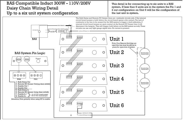
The wiring of the Induct BAS compatible unit as a part of a facilities BACnet protocol is done simply by wiring the units in a series as shown in the above image. It is important to maintain that each wire is routed to the correct location in each port.
