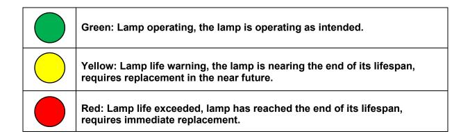
When the "Lamp Operating" LED color is yellow indicating "Lamp Life Warning" please contact your local distributor or an Air Sniper representative directly for a replacement. The Induct BAS compatible unit is designed as a complete unit, therefore when the lamp expires, the entire unit must be replaced.
