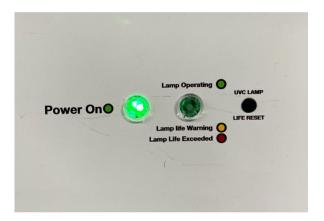
6. Once an airflow is detected, the UV Lamp will illuminate, and the "Lamp Operating" LED will turn on.
