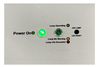
6. Once an airflow is detected, the UV Lamp will illuminate, and the "Lamp Operating" LED will turn on.
