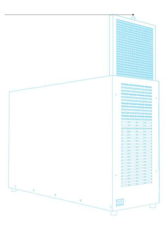
Run the filter under warm water making sure to rinse them in reverse of the air flow (refer to the arrow) so that the water can push the particles out. As the water runs through the filter, wipe the bottom with a wet cloth. DO NOT SUBMERGE THE FILTER.
